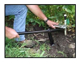
The angle iron on the bottom of the jack helps to keep it from sliding on ridges.
