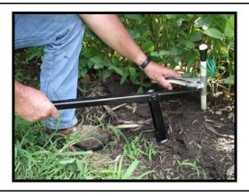
If sensor does not pull easily, and to avoid damage, pour water in a hole that is dug next to the sensor shaft.
